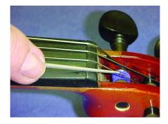
Use large end of rat tail file to widen grooves (careful not to deepen the grooves). Ideally, strings should have at least 1/3 their diameter above the top of the bridge and nut.
