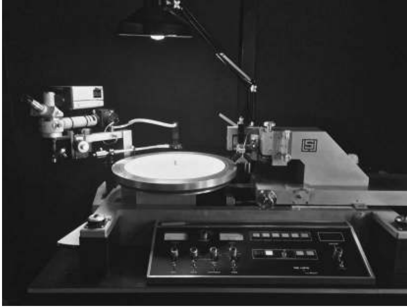
Figure 1.1 A disc-cutting lathe.
